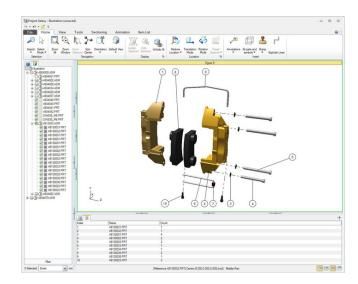
Leverage CAD product structures to dynamically generate parts lists with call outs and maintain associativity with engineering model to automate changes when product design changes occur.
